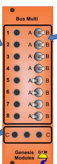
Selection switches – Route the socket to either an 'A' or a 'B' bus.
